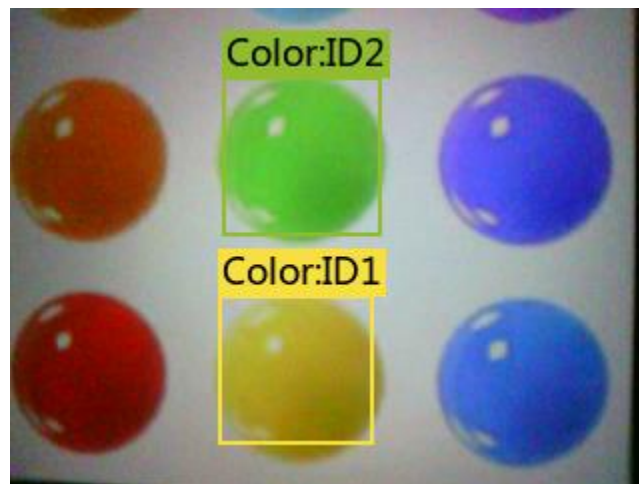
Figure 8: Color Recognition After It Was Previously Learned by The Camera Sensor (Permission requested from DFRobot)
