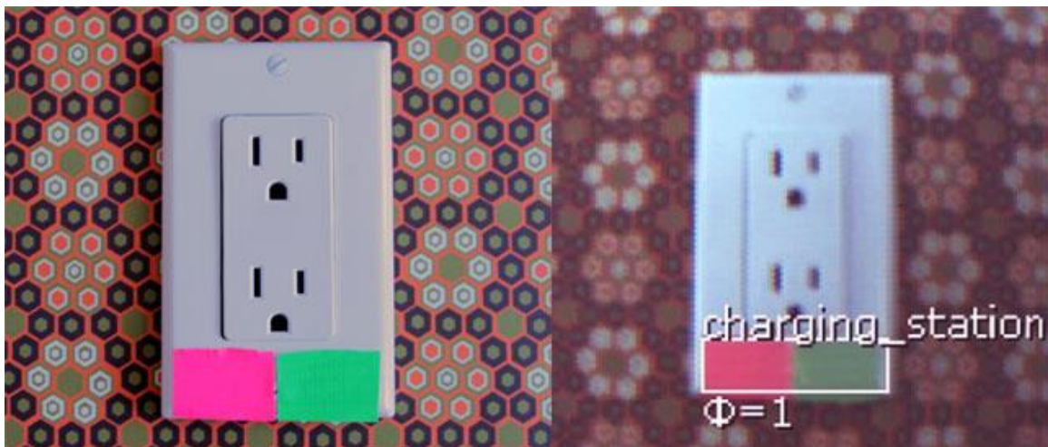
Figure 9: Color Code Tag Detected and Recognized by Pixy2 (Permission Requested From Charmed Labs and Carnegie Mellon)
